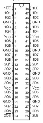
These devices can be used as two 8-bit latches or one 16-bit latch. When the latch-enable (LE) input is high, the Q outputs follow the data (D) inputs. When LE is taken low, the Q outputs are latched at the levels set up at the D inputs.
